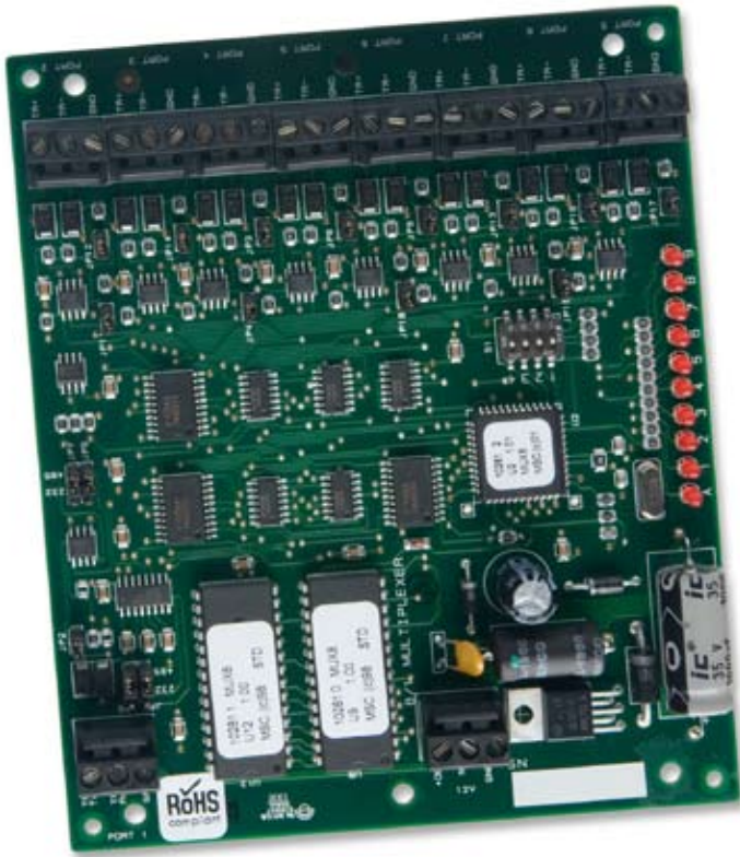
The MUX-8 is an 8-port multiplexer that can multiplex eight 2-wire RS-485 communication channels
