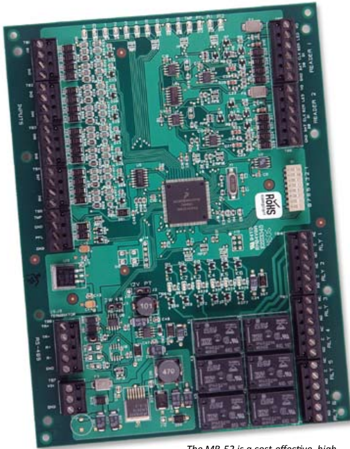
The MR-52 is a cost-effective, high-performance dual reader I/O module.
